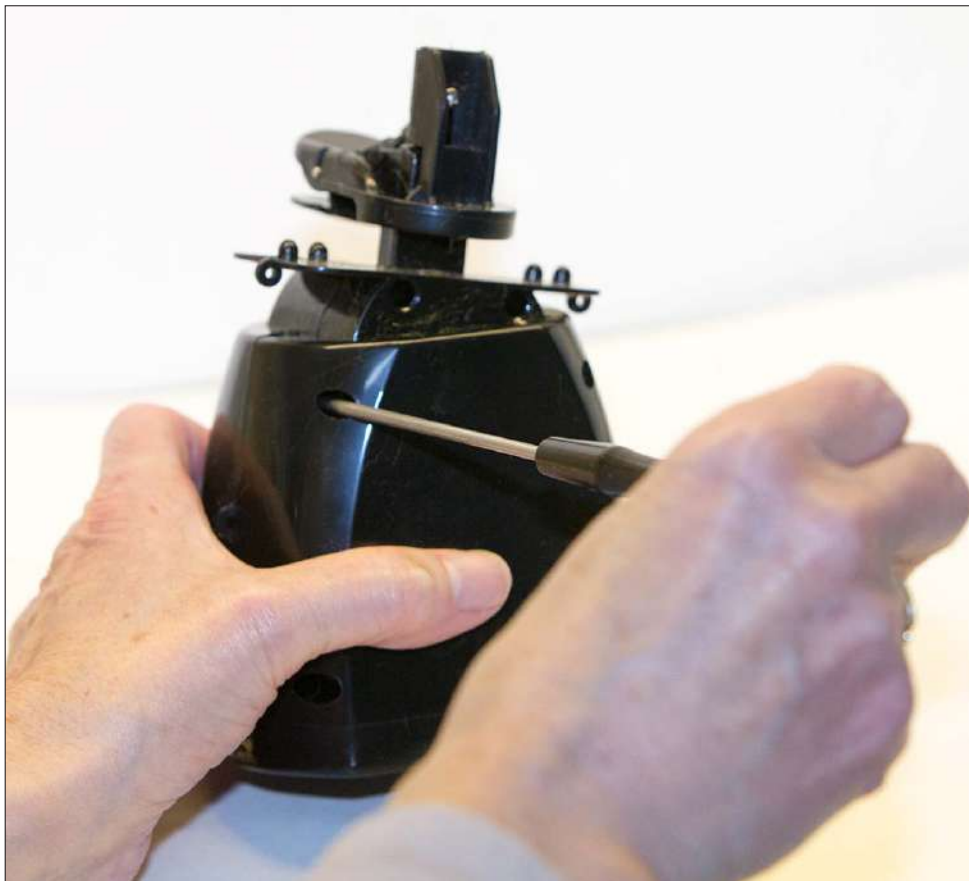
FIGURE 10-2: Removing the case of the movement mechanism.
