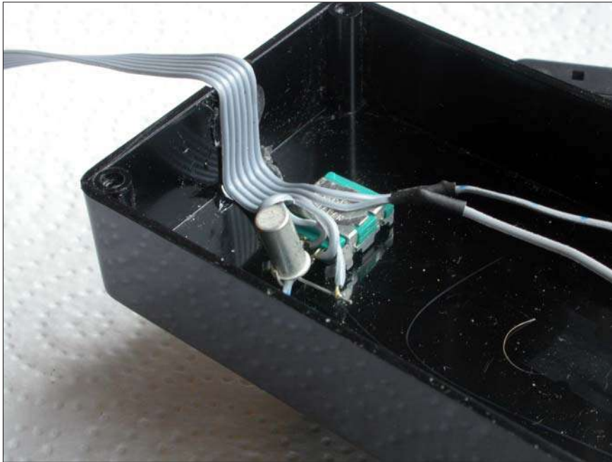
FIGURE 15-5: The wiring for the roto-sketch control box.
